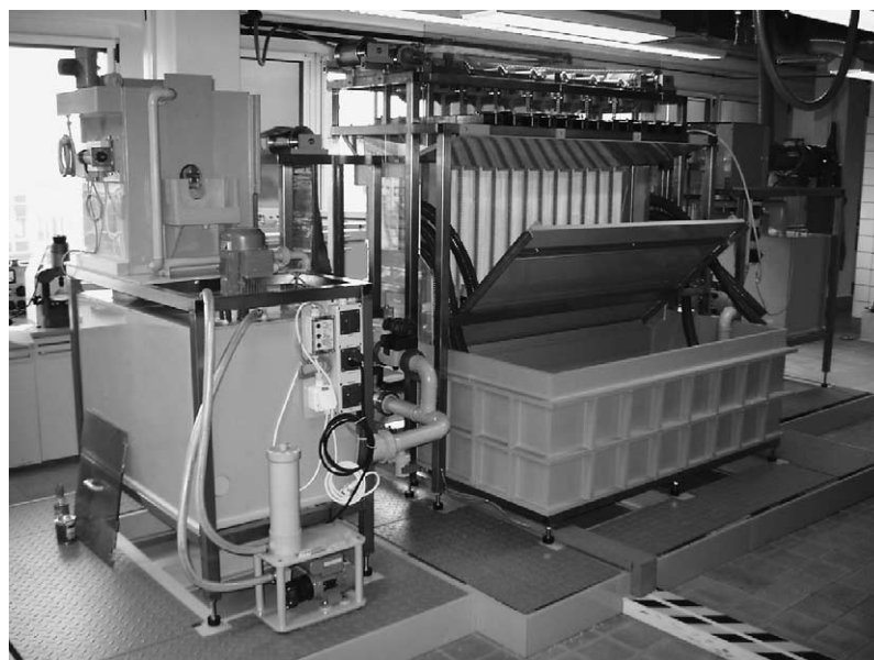
Fig. 2. Pilot plant for continuous electroforming and galvanizing process to produce lead grid strip.
